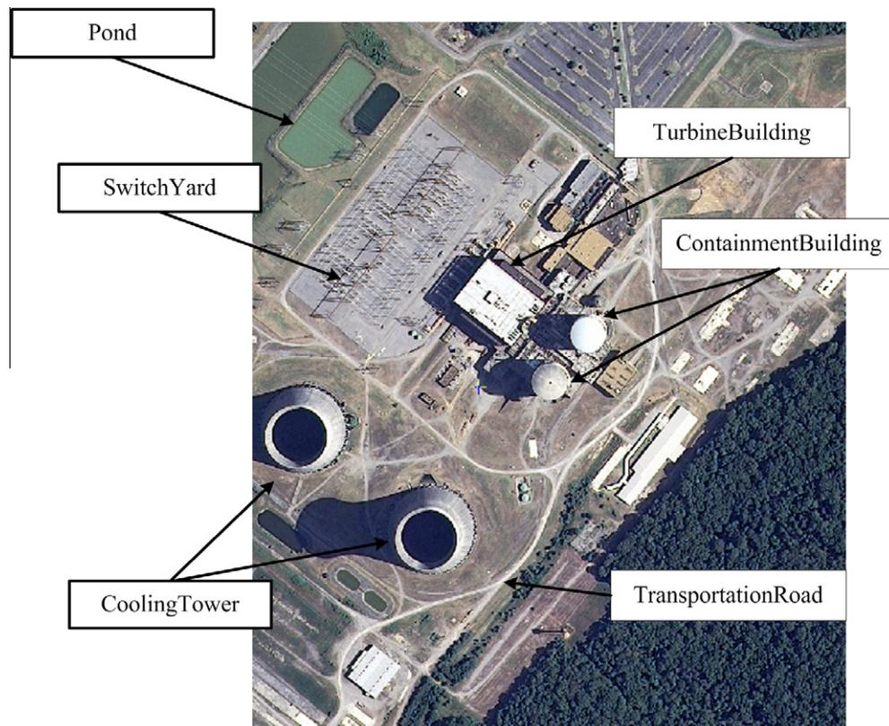
Fig. 2. An example of a nuclear power plant.
